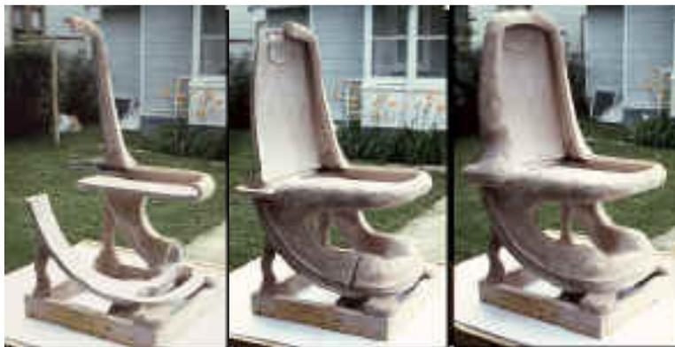
The mold matrix is bonded together temporarily, using bandage size plaster soaked hemp swatches to hold the mold together during the curing of attachment joints of the FRP part encased in the mold matrix. This acts like a cocoon and is very strong, effective and easy to remove, for de-molding the enclosed monocoque composite part.
