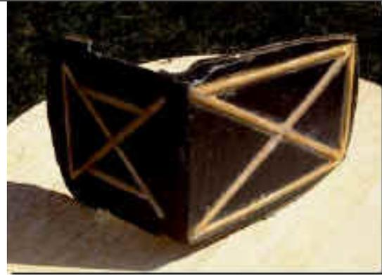
**Constructed of carbon graphite with laminated balsa stiffeners**
