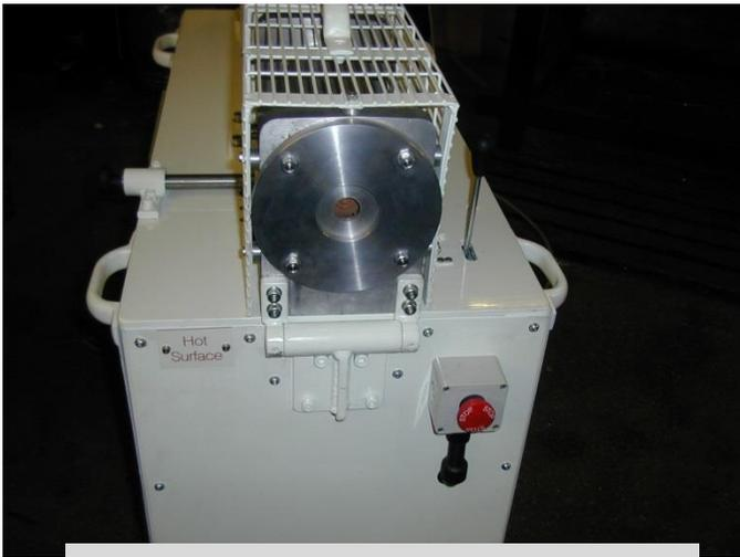
Remove 4 nuts to Interchange Die Plate
