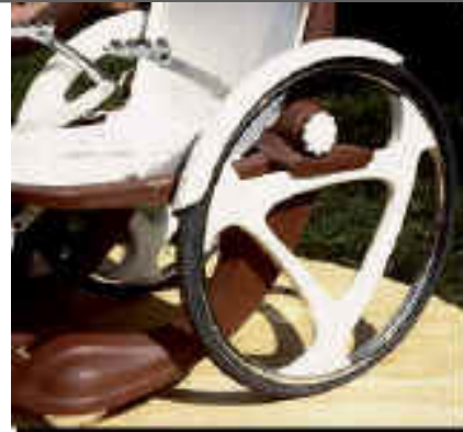
Adjustable armrest linkage, seating carrier insert, and adjustable pylon mount
