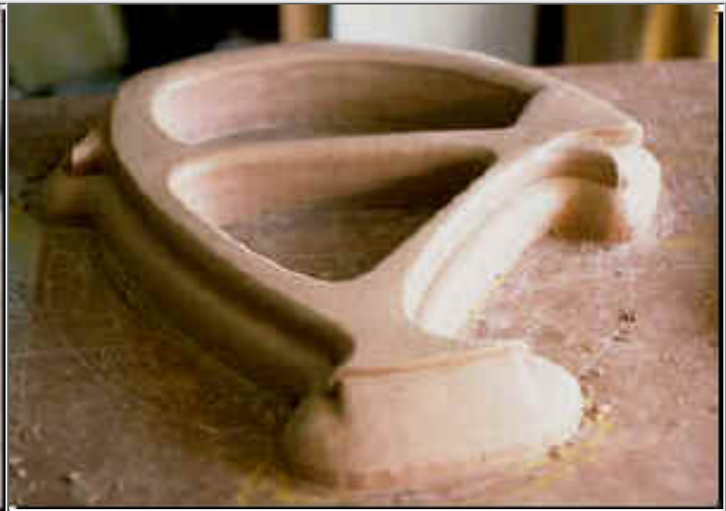
Adding runoff to model provides easy access for hand laying up of FRP part (Fiber Reinforced Plastic)
