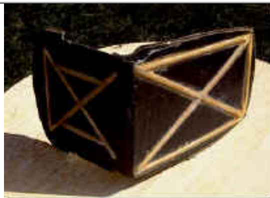
Constructed of carbon graphite with laminated balsa stiffeners
