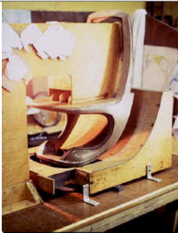
Clay model becomes removable by detaching it from its seat armature stanchion
