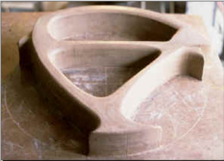
Model is thicker, allowing the integrated removable fender option included into one model design. 1/8" thick masonite profile is used as contact area base plate for modeling of the spoke-less wheel design.
