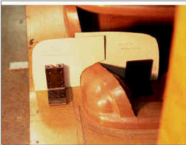
Master right side, and the making of a cardboard template
