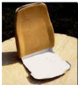
The seating carrier insert is a holding fixture, keeping the seating cushion in design alignment with the wheelchair mounting attachment points
