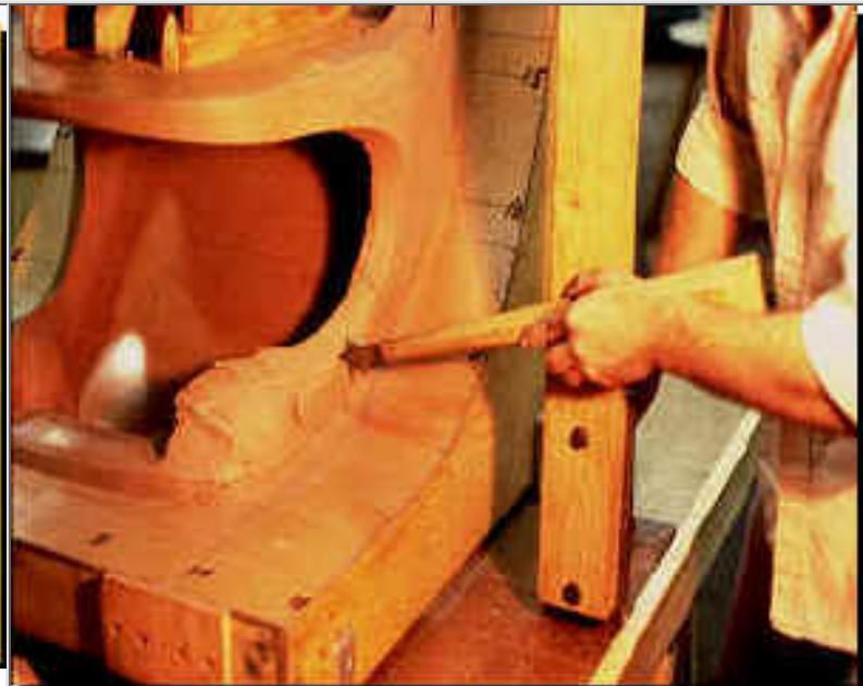
Marking a locating line for the template
