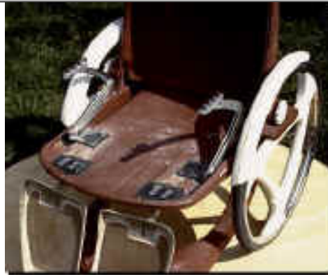
Bonded-in attachment brackets for arm rest and calf support mounting points
