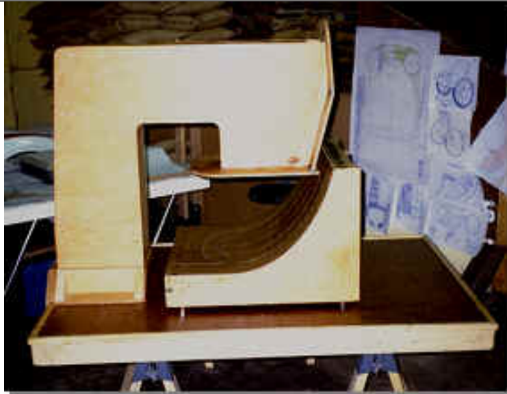
Seat armature stanchion with profiled modeling platform installed
