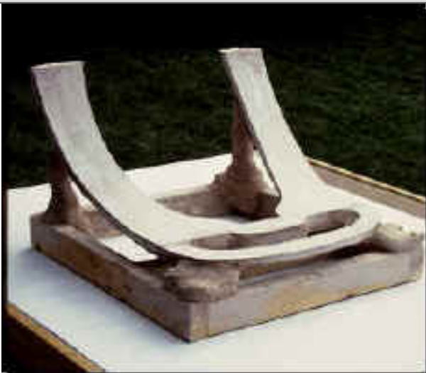
Mold alignment base: Allows for the precise alignments of all mold components
