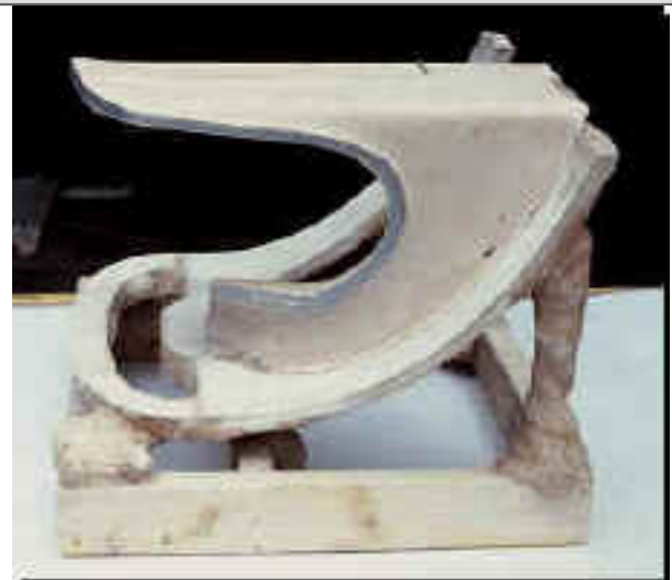
Inner left mold component, nesting on alignment base
