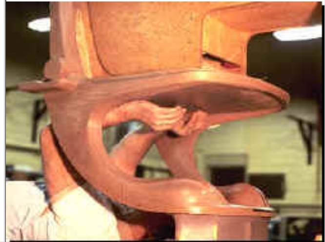
Clay model becomes removable by detaching it from its seat armature stanchion
