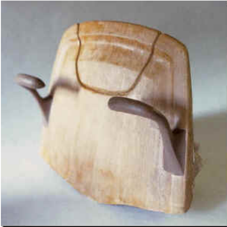
Plaster modeling substrate / Hand grips modeled on seat-back plaster substrate
