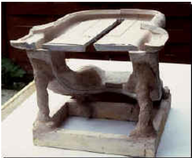
Left and right, inner and outer mold components, with center key section removed. The key section permits the inner mold components to be removed during the de-molding of the final assembled part
