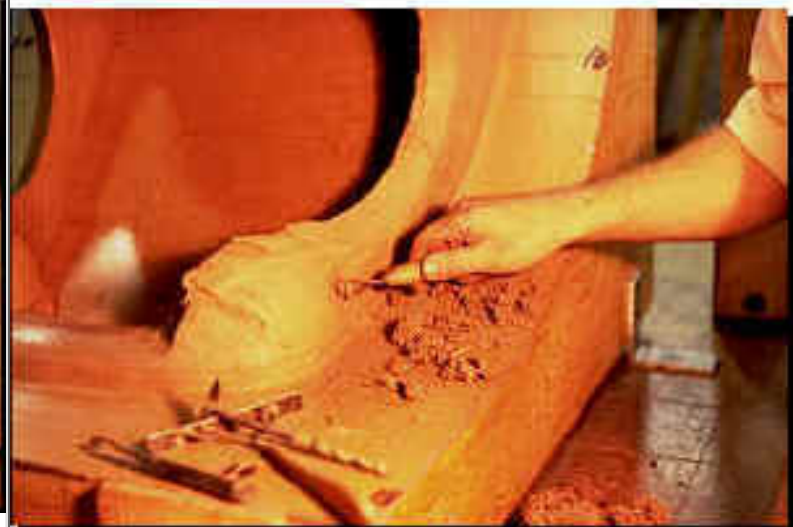
Filling between tempered sections and finishing the model surface between the sections. Repeat process until left side is reproduced from the right side of the master model.
